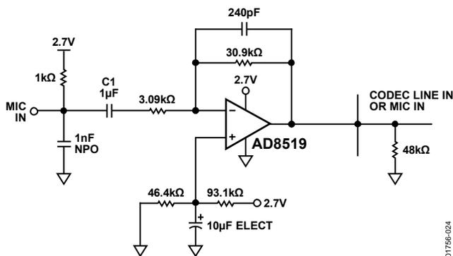
Figure 24. 10× Microphone Preamplifier
