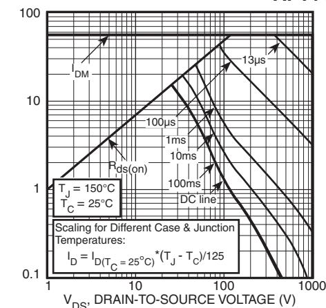
Figure 10, Maximum Forward Safe Operating Area
