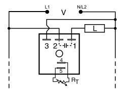
R<sub>+</sub> is used when external adjustment is ordered.
