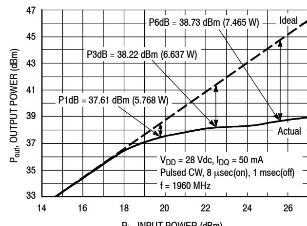
Figure 8. Pulsed CW Output Power versus Input Power
