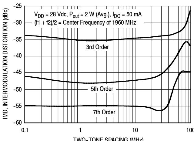
Figure 7. Intermodulation Distortion Products versus Tone Spacing
