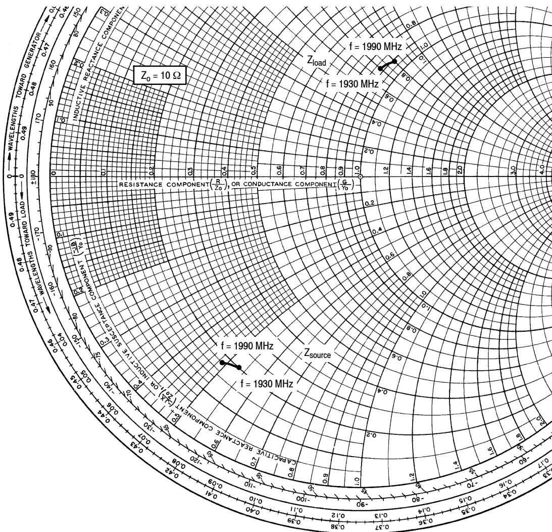
$V_{DD} = 28 \text{ Vdc}, I_{DQ} = 50 \text{ mA}, P_{out} = 4 \text{ W PEP}$
