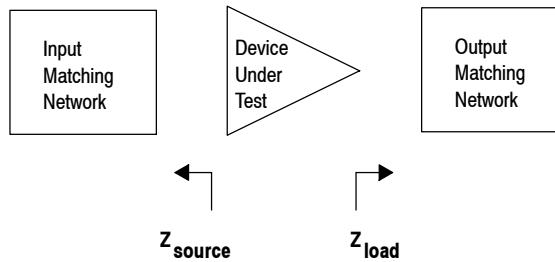
Figure 13. Series Equivalent Source and Load Impedance
