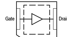
Note: The center pad on the backside of the package is the source terminal for the transistor.
