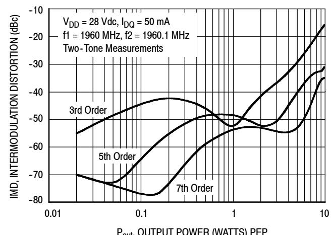
Figure 6. Intermodulation Distortion Products versus Output Power
