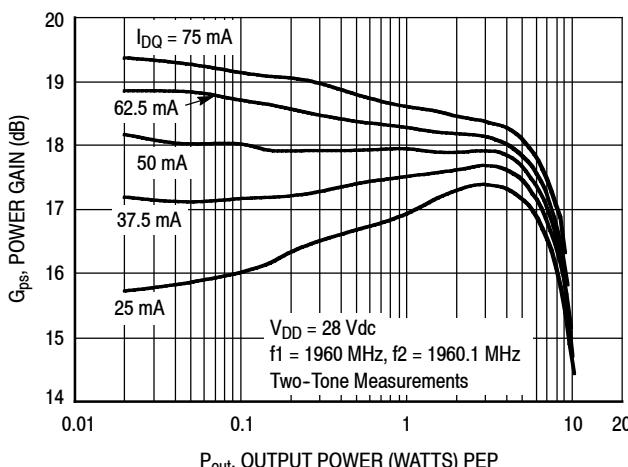
Figure 5. Two-Tone Power Gain versus Output Power
