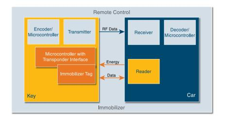
Bi-directional RF link for RKE functions as well as for the extremely secure duplex RF link in a Passive Entry Go (PEG) system. The LF link is used for the wake-up channel in a PEG system as well as for the immobilizer function to start the RF communication.
