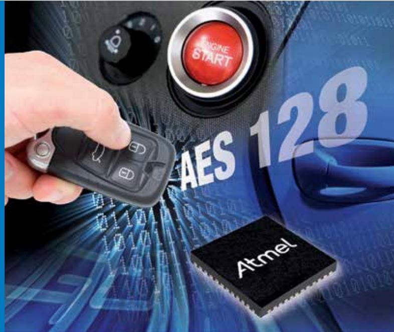
Uni-directional RF link for the keyless entry function to open or lock car doors. The immobilizer system is built with a bi-directional LF link operating with the AUT64 crypto algorithm.
