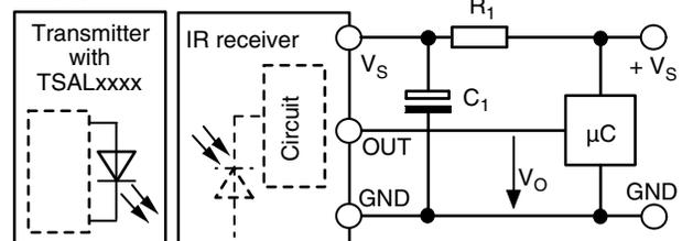
The external components  $R_1$  and  $C_1$  are optional to improve the robustness against electrical overstress (typical values are  $R_1 = 100 \Omega$ ,  $C_1 = 0.1 \mu\text{F}$ ).
