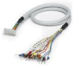
Assembled, shielded round cable with a 16-pos. socket strip and an open end. At the open end, the wires are labeled 1 to 16 and are fitted with ferrules, shield connection at open end, cable length: 17 m
