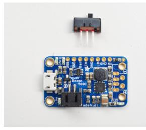
The switch will go into the breakout header, and attach to **VBAT EN** and **GND**
