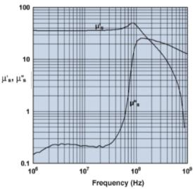
Measured on an 19/10/6mm toroid using the HP 4284A and the HP 4291A.
