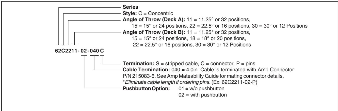
Custom custom shaft, pushbutton actuation force and termination options are available.
