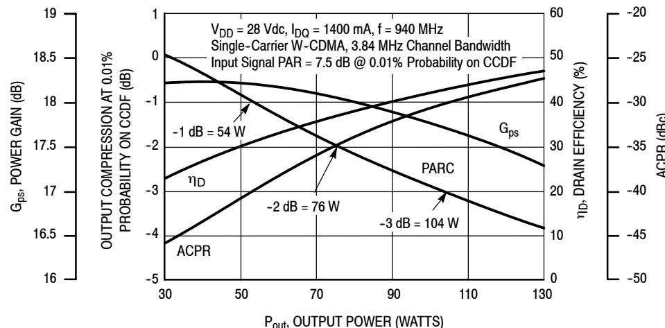
Figure 4. Output Peak-to-Average Ratio
