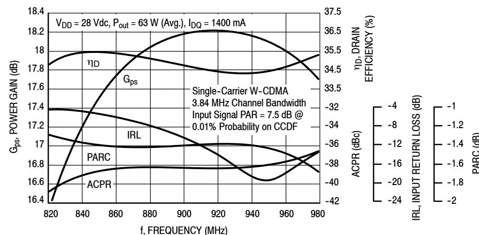
Figure 2. Output Peak-to-Average Ratio Compression (PARC)
