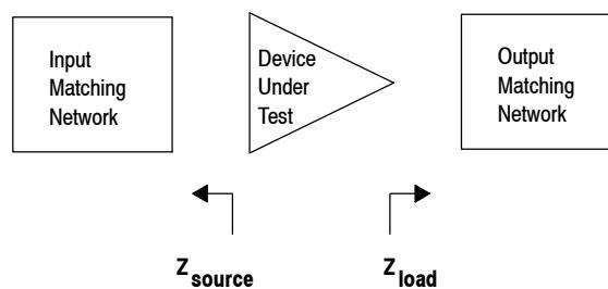
Figure 9. Series Equivalent Source and Load Impedance
