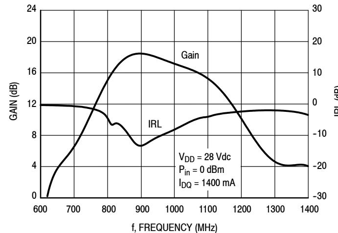
$V_{DD} = 28$  Vdc,  $I_{DQ} = 1400$  mA,  $P_{out} = 63$  W Avg.
