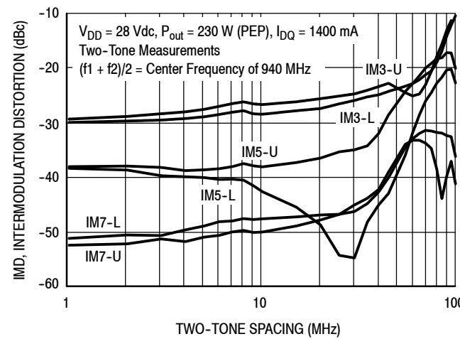
Figure 3. Intermodulation Distortion Products
