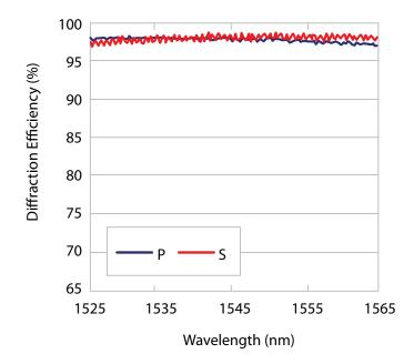
LightSmyth Technologies' transmission gratings are fabricated on fused silica substrates and robust dielectric films by state-of-the-art projection photolithography and reactive ion etch. These high fidelity semiconductor fabrication methods enable precise realization of sophisticated proprietary grating designs that provide diffraction efficiency close to 100% and line spacing control to 1 part per million.
