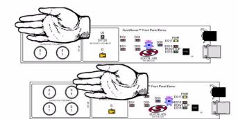
Press the capacitive sensing pads S1-S4 on the board. Each will light a corresponding red LED when firmware senses a finger's presence.
