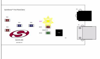
4 Move a hand in close proximity to the area of the board labeled "CAPACITIVE PROXIMITY." The blue LED DS5 turns on. Move in close proximity to the area labeled "INFRARED PROXIMITY." The blue LED DS6 turns on.
