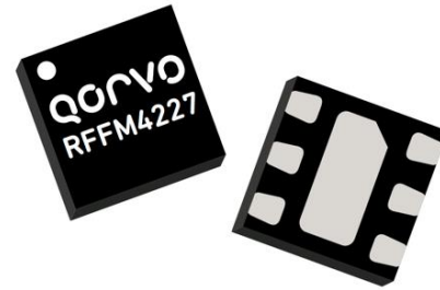
6 Pad 1.6 x 1.6 mm DFN Package
