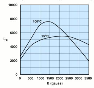
Measured on an 18/10/6mm toroid at 10kHz.
