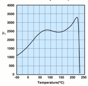
Measured on an 18/10/6mm toroid at 100kHz.
