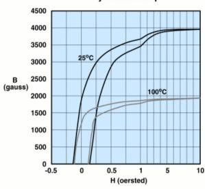
Measured on a 17/10/6mm toroid at 10kHz.
