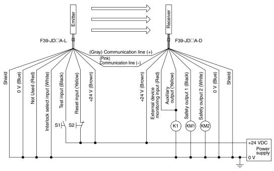
S1 : External test switch (connect to 0 V if a switch is not required)
