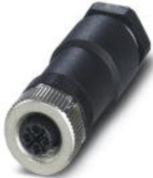
Connector, 4-position, Socket straight M12, S-coded, Screw connection, Knurl material: Zinc die-cast, nickel-plated, Cable gland Pg11, External cable diameter 8 mm ... 10 mm
