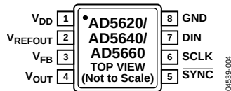
Figure 4. MSOP Pin Configuration
