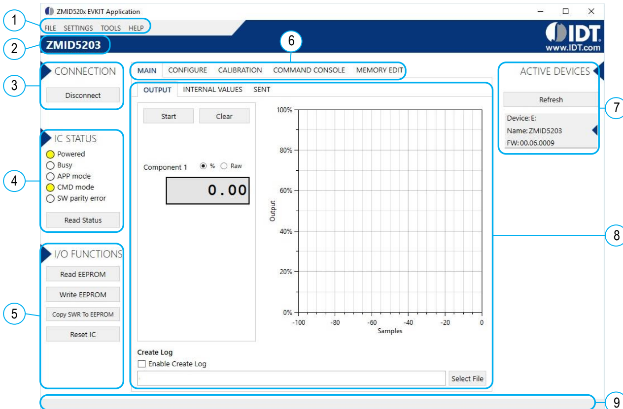
Figure 7. Sections of the GUI Display – Example ZMID5203
