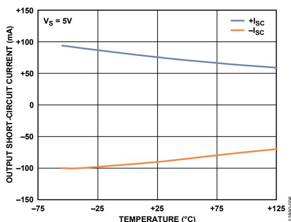
Figure 6. Output Short-Circuit Current vs. Temperature (5 V)
