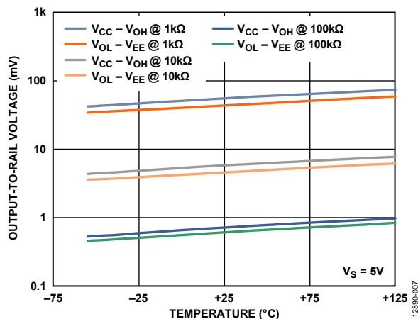
Figure 7. Output-to-Rail Voltage vs. Temperature (5 V)
