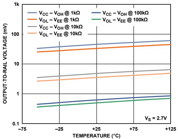
Figure 4. Output-to-Rail Voltage vs. Temperature (2.7 V)
