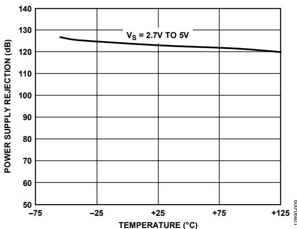
Figure 9. Power Supply Rejection vs. Temperature
