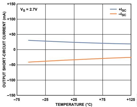
Figure 3. Output Short-Circuit Current vs. Temperature (2.7 V)
