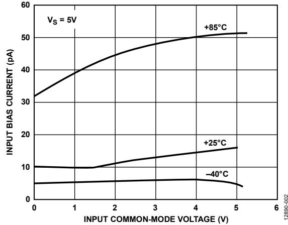
Figure 2. Input Bias Current vs. Input Common-Mode Voltage
