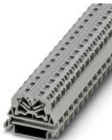
Mini feed-through terminal block, Connection method: Spring-cage connection, Cross section: 0.08 mm 2 - 4 mm 2 , AWG: 28 - 12, Width: 10.4 mm, Height: 22 mm, Color: blue, Mounting type: NS 35/7,5, NS 35/15
