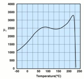
Measured on an 18/10/6mm toroid at 100kHz.
