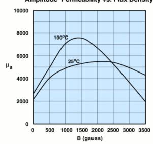
Measured on an 18/10/6mm toroid at 10kHz.
