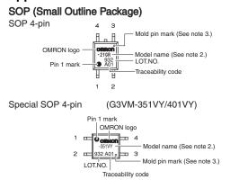
Note: 1. The actual product is marked differently from the image shown here. Note: 2. "G3VM" does not appear in the model number on the Relay.
