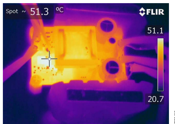
Figure 15. Thermal Image of the ADP1071-1 at 48\text{ V}_{\text{DC}} Input, Full Load, No Airflow, and 0.5 Hour Soaking Time
