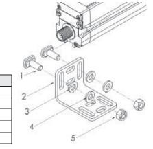
Note: Shipments contain a different quantity of brackets, depending on the length of the light grid. Longer light grids contain a higher number of brackets, following the rule of one bracket every 400 mm.
