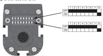
Note: There are two lines of dip switches in each transmitter and receiver. The settings must be done for both lines. Change the setting of the dip-switch and close the cap again. The light grid can now be reconnected to the power supply.
