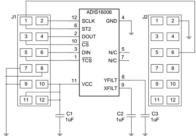
Figure 1 - ADIS16006/PCB Schematic
