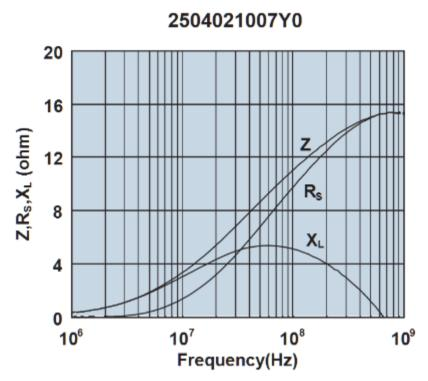
Impedance, reactance, and resistance vs. frequency.
