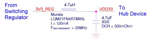
Figure 2.2 Example Switching Regulator Noise Filter
