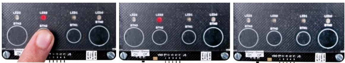
Figure 3-13. Test Sequence for Delay Off Feature
