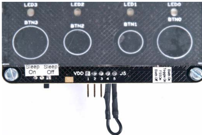
Figure 3-20. BTN1 Sensor Shorted to Ground
