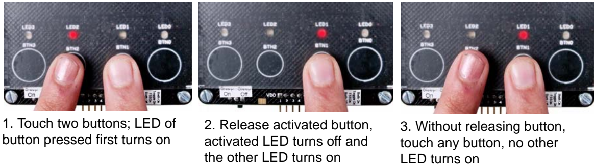
Figure 3-7. FSS Feature Test Sequence
