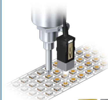
LED potting shape measurement
