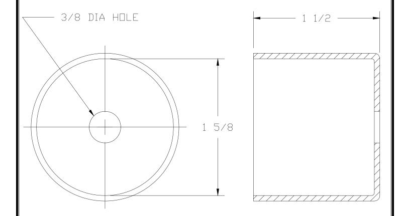
Recommended especially for 110Vac & 250Vac models, or any other classic ('SC') Sonalert  $^{\tiny{(8)}}$  model where terminal insulation is desired.
