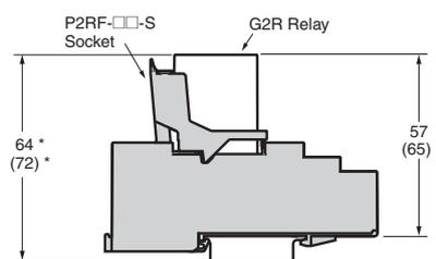
Figures of height in ( ) is with G2R Relays with Latching Levers.
