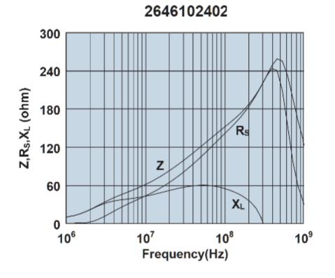
Impedance, reactance, and resistance vs. frequency.
