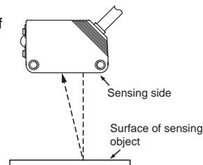
If the sensing object has a glossy surface, however, incline the Sensor by 5° to 10° as shown in the illustration, provided that the Sensor is not influenced by background objects.
