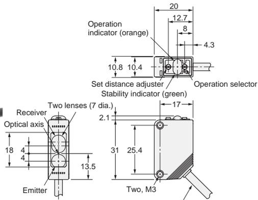
4-dia., vinyl-insulated round cable with 4 conductors (Conductor cross section: 0.2 mm<sup>2</sup> (AWG24); Insulator diameter: 1.1 mm), Standard length: 2 m/0.5 m
