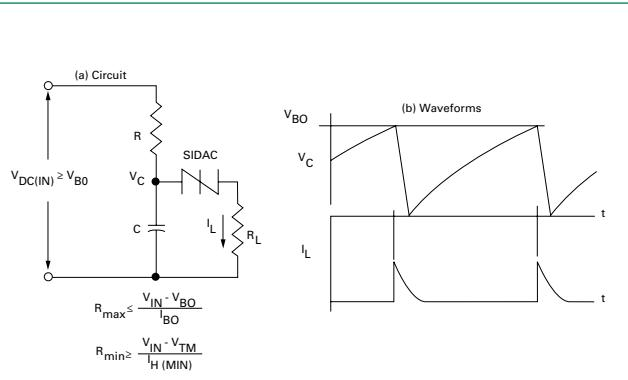
**Figure 14: Low-voltage Input Circuit for Gas Ignition**
