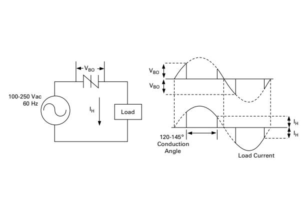
**Figure 13: Relaxation Oscillator Using a SIDAC**
