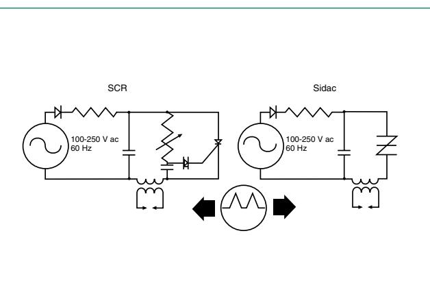
**Figure 16: Xenon Lamp Flashing Circuit**
