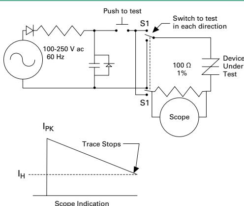
**Figure 12: Basic SIDAC Circuit**
