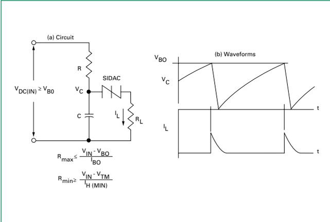
**Figure 14: Low-voltage Input Circuit for Gas Ignition**
