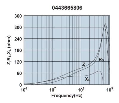
Impedance, reactance, and resistance vs. frequency.
