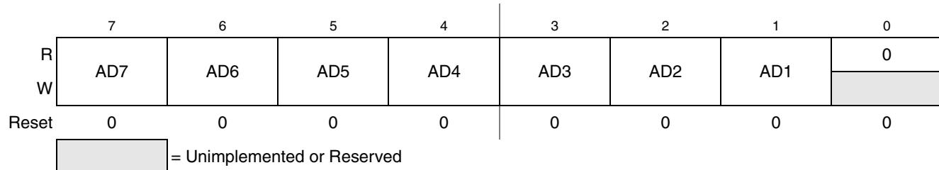
Figure 11-3. IIC Address Register (IICA)
