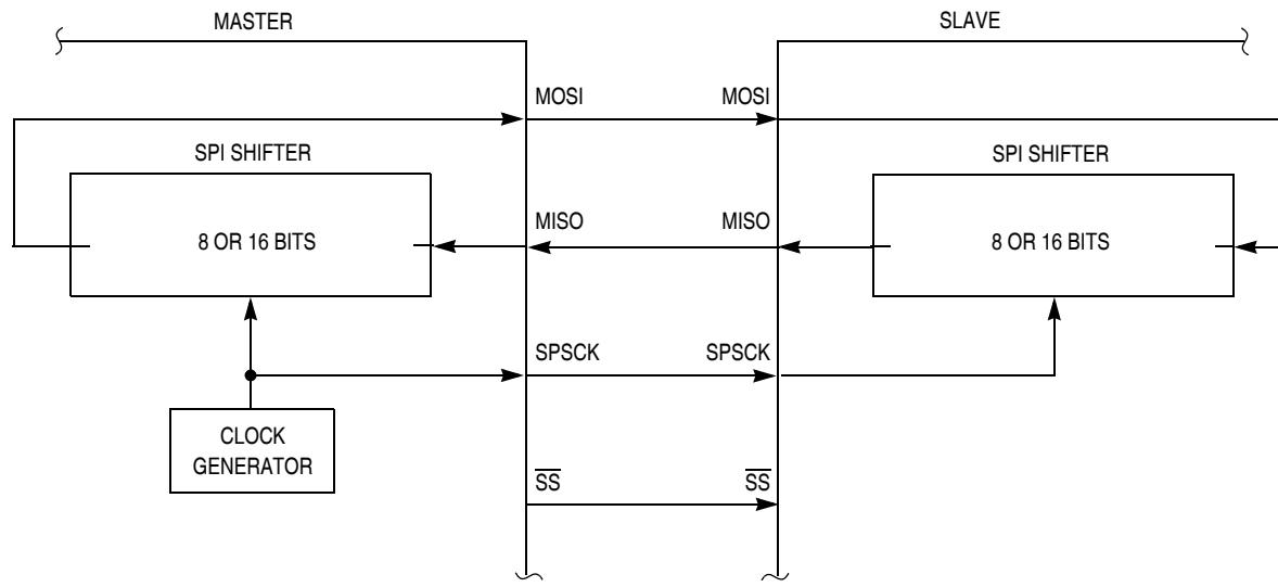
Figure 15-3. SPI System Connections
