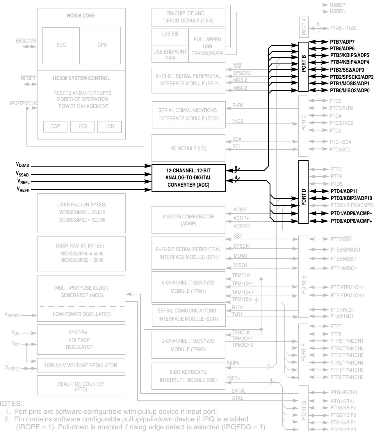
Figure 10-1. MC9S08JM60 Series Block Diagram Highlighting ADC Block and Pins
