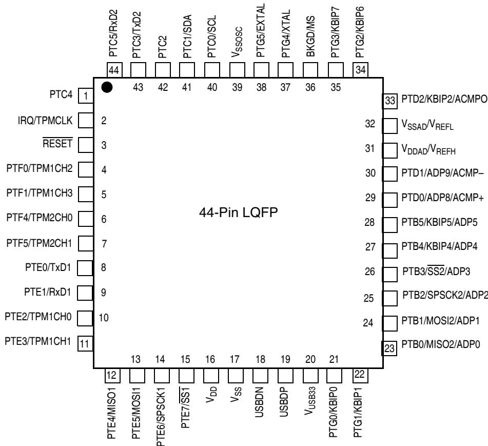
Figure 2-3. MC9S08JM60 Series in 44-Pin LQFP Package
