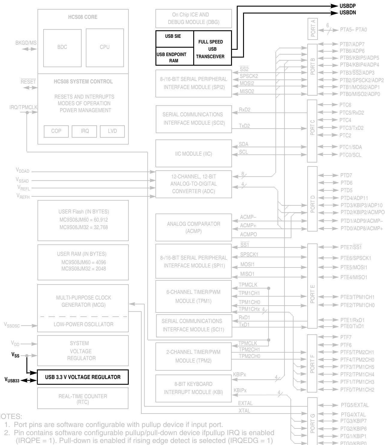
Figure 17-1. MC9S08JM60 Series Block Diagram Highlighting USB Blocks and Pins
