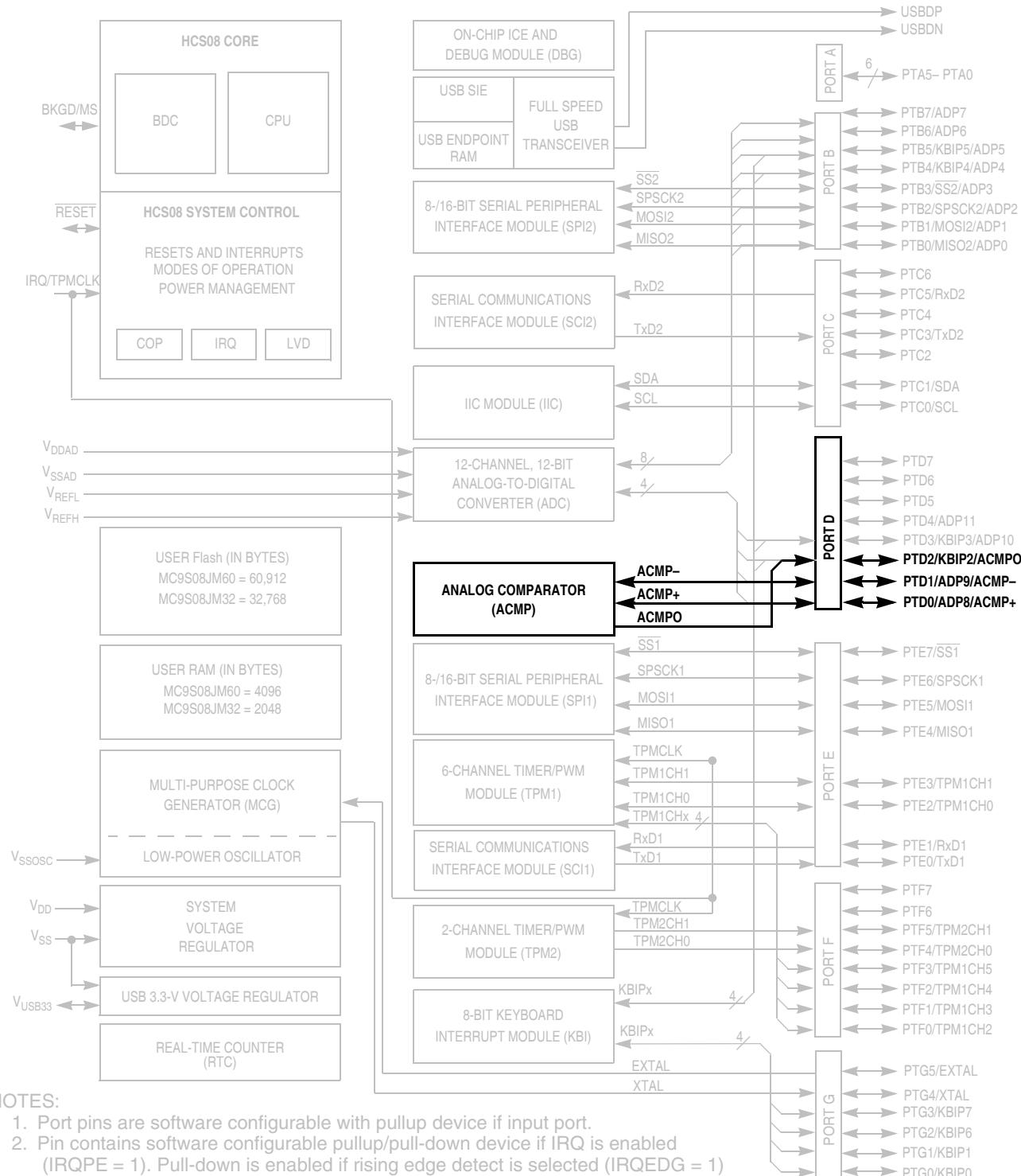
Figure 8-1. MC9S08JM60 Series Block Diagram Highlighting ACMP Block and Pins
