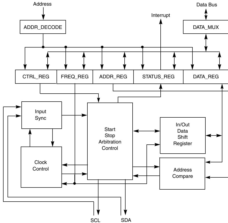
Figure 11-2. IIC Functional Block Diagram
