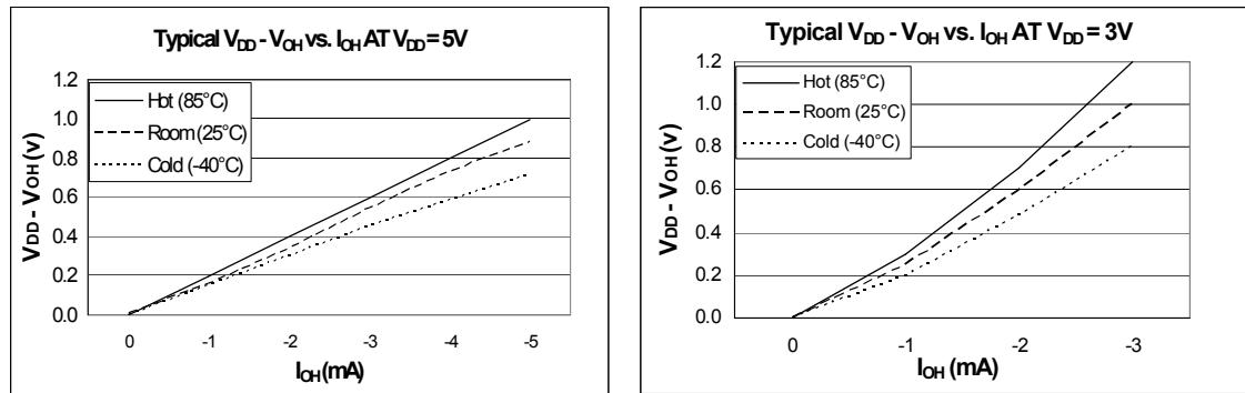
Figure A-4. Typical High-side Drive (source) characteristics – Low Drive (PTxDs<sub>n</sub> = 0)
