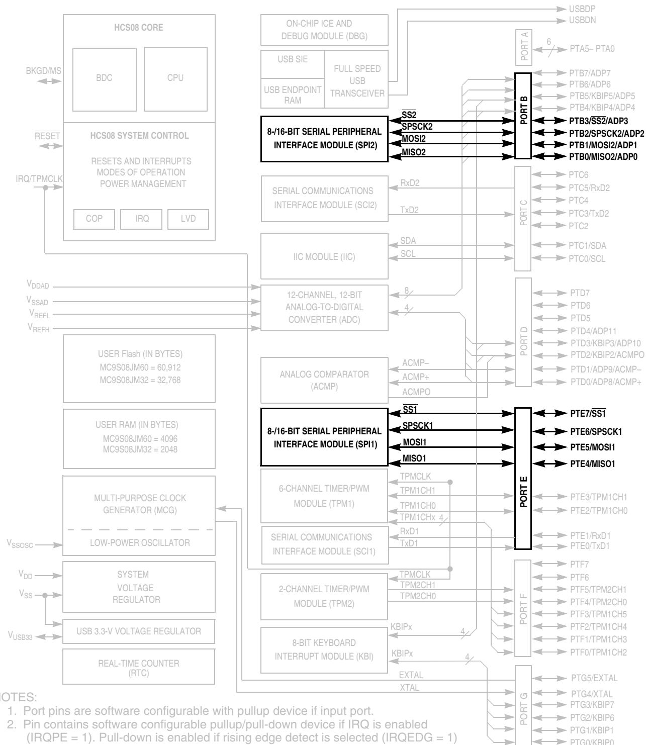
Figure 15-1. MC9S08JM60 Series Block Diagram Highlighting the SPI Blocks and Pins
