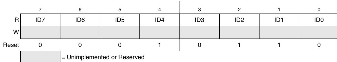
Figure 5-8. System Device Identification Register — Low (SDIDL)
