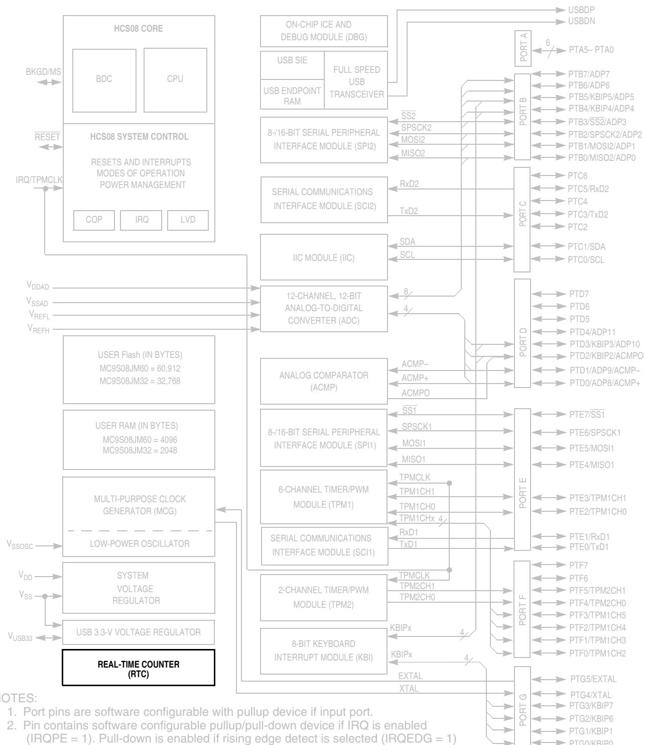
Figure 13-1. MC9S08JM60 Series Block Diagram Highlighting RTC Block
