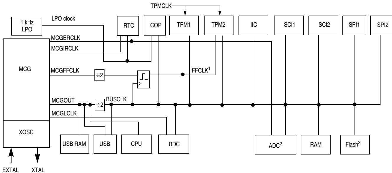
1. The FFCLK is internally synchronized to the bus clock and must not exceed one half of the bus clock frequency.
