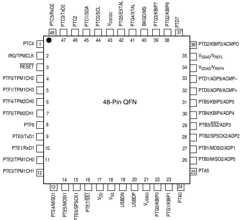
Figure 2-2. MC9S08JM60 Series in 48-Pin QFN Package
