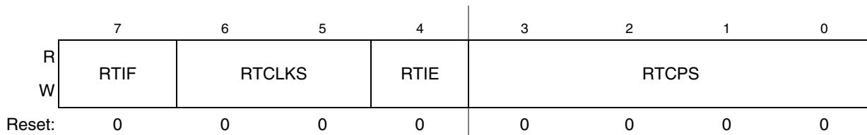
Figure 13-3. RTC Status and Control Register (RTCSC)
