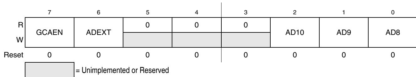
**Figure 11-8. IIC Control Register (IICC2)****Table 11-8. IICC2 Field Descriptions**
