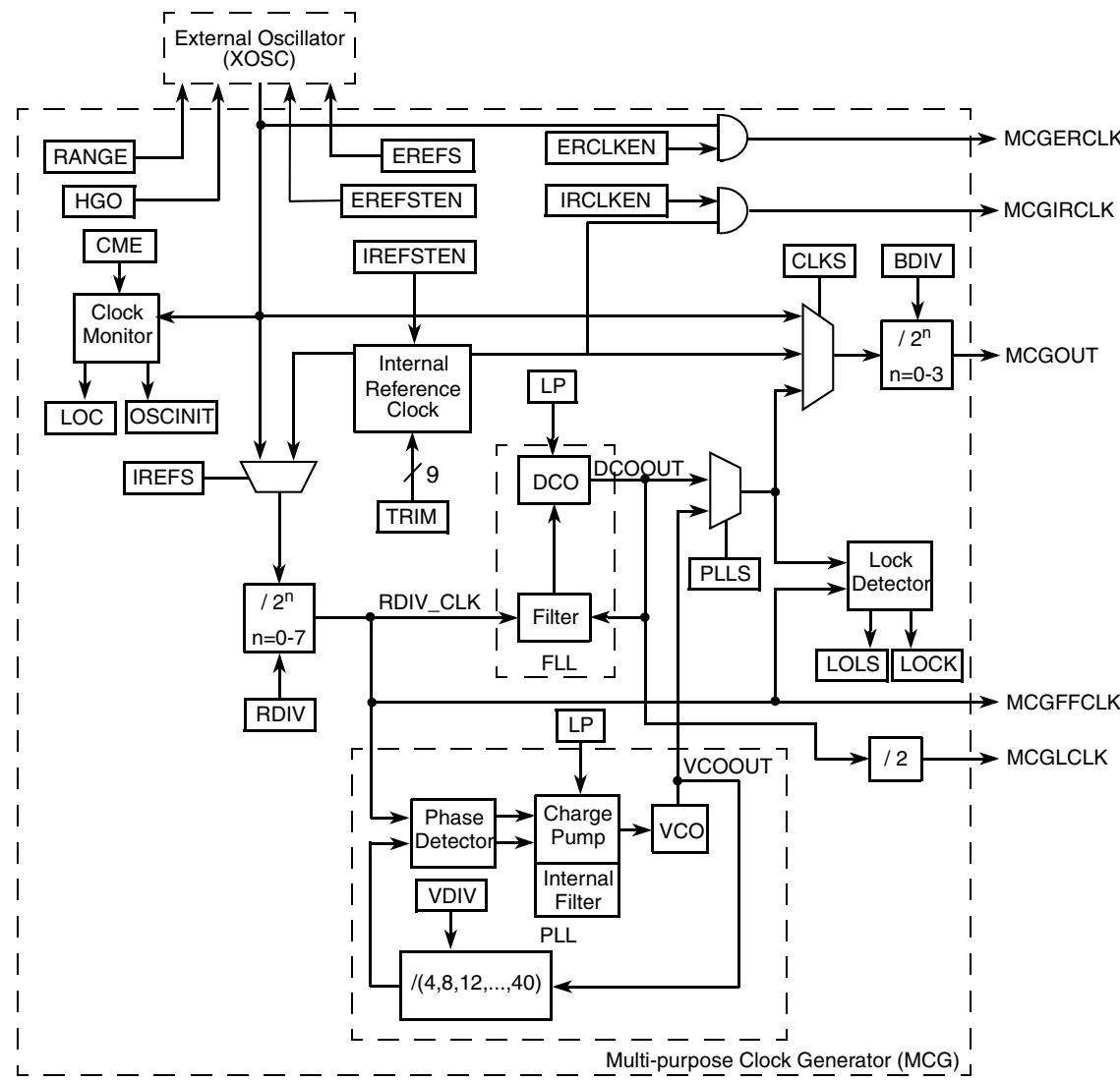
Figure 12-2. Multi-Purpose Clock Generator (MCG) Block Diagram
