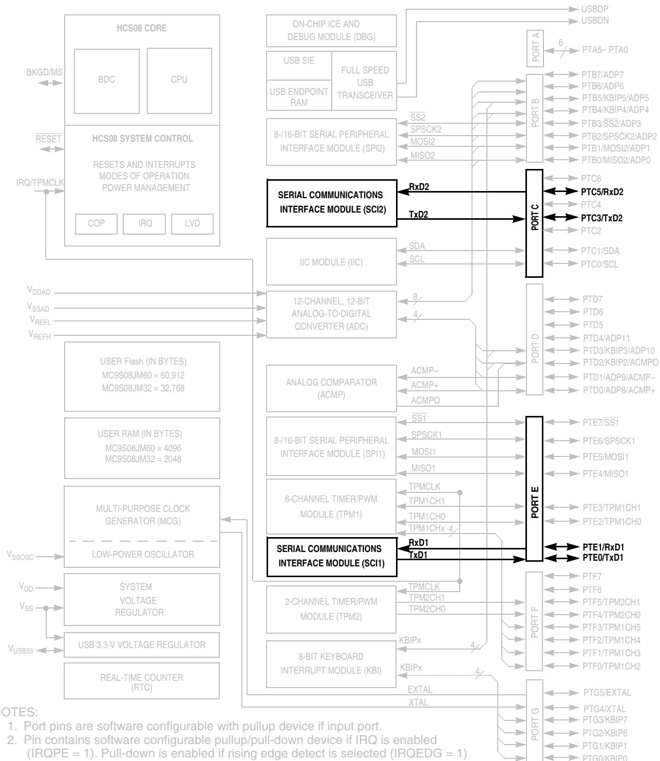
Figure 14-1. MC9S08JM60 Series Block Diagram Highlighting the SCI Blocks and Pins
