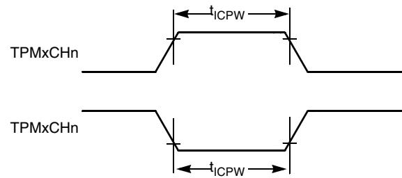
Figure A-9. Timer Input Capture Pulse
