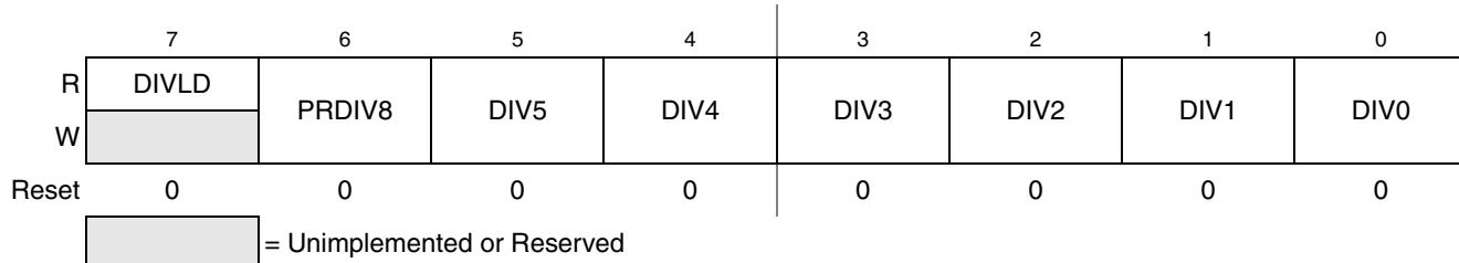
Figure 4-5. Flash Clock Divider Register (FCDIV)
