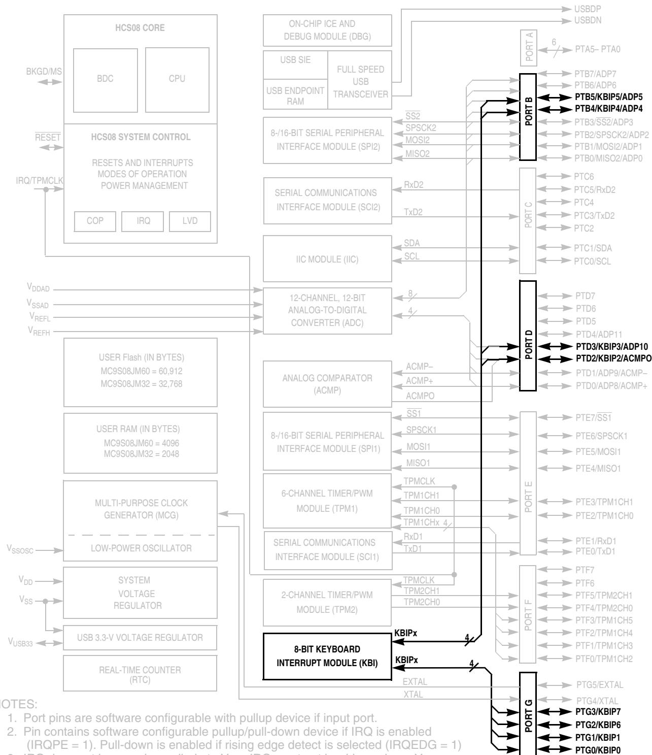
Figure 9-1. MC9S08JM60 Series Block Diagram Highlighting KBI Block and Pins
