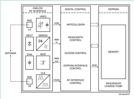
Fig 1. Block diagram of ICODE SLIX-S
