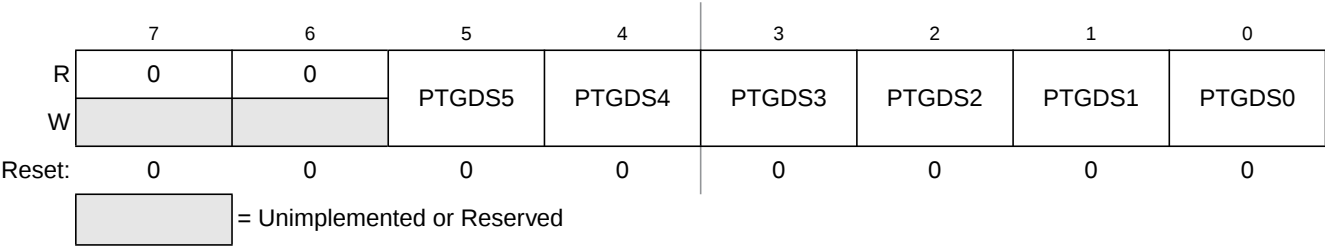
Figure 6-46. Drive Strength Selection for Port G Register (PTGDS)
