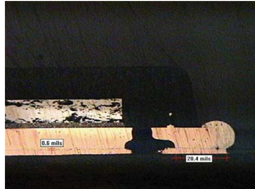
37% Paste coverage, Encroached Via, 0.6 mil Standoff
