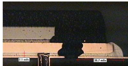
81% Paste Coverage, Encroached Via, 2.1 mil Standoff
