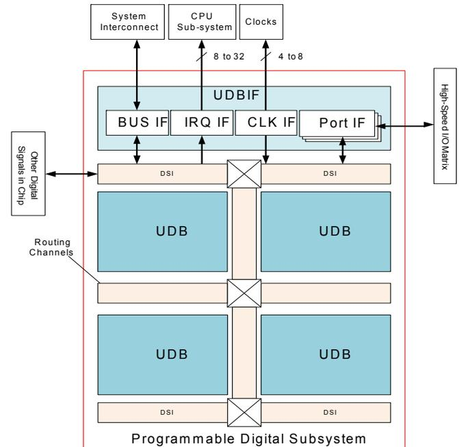
UDBs can be clocked from a clock divider block, from a port interface (required for peripherals such as SPI), and from the DSI network directly or after synchronization.
