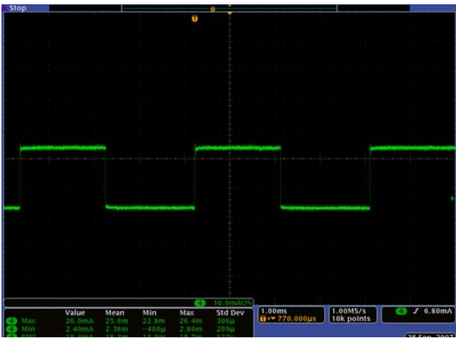
FIGURE 13. I LED AT 50% PWM DIMMING
