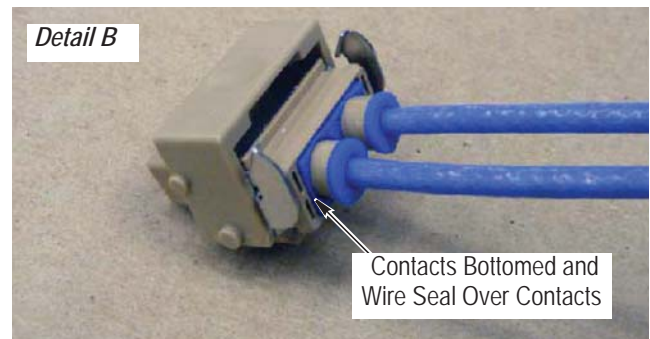
Mating Face of Plug Connector
