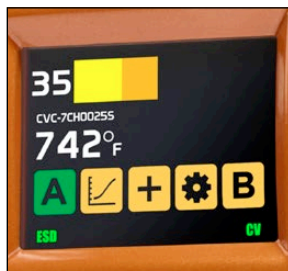
Tip temperature displayed on large color screen.
