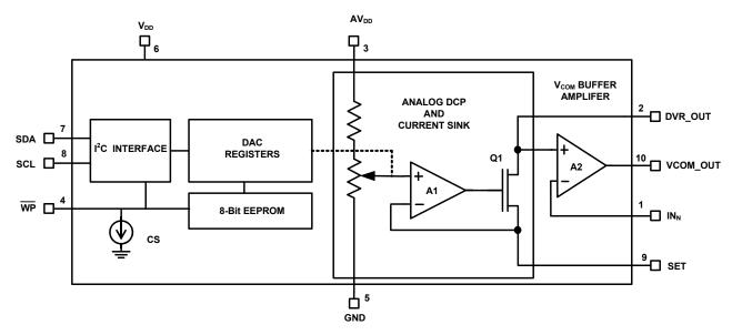
FIGURE 2. BLOCK DIAGRAM OF THE ISL24211
