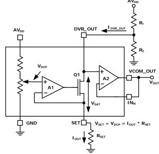
FIGURE 5. CURRENT SINK CIRCUIT
