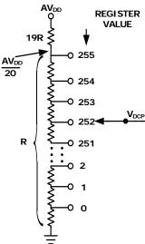
FIGURE 4. SIMPLIFIED SCHEMATIC OF DCP
