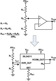
FIGURE 3. MECHANICAL ADJUSTMENT REPLACEMENT
