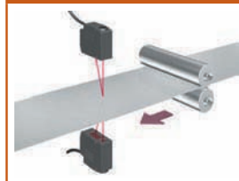
Measuring Electrode Thickness on Dielectrics
