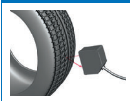
Measuring Tire Exteriors
